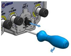
Bend the screwdriver slightly and pull out the unit using the tilt adjustment wheel.
