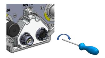
Slot the unit into the antenna and tighten the screw with 2,7±0,3 Nm using a screwdriver T20. Remove protection caps and connect the AISG-cable(s) as required. Protection caps shall remain on connectors not connected to cables.
